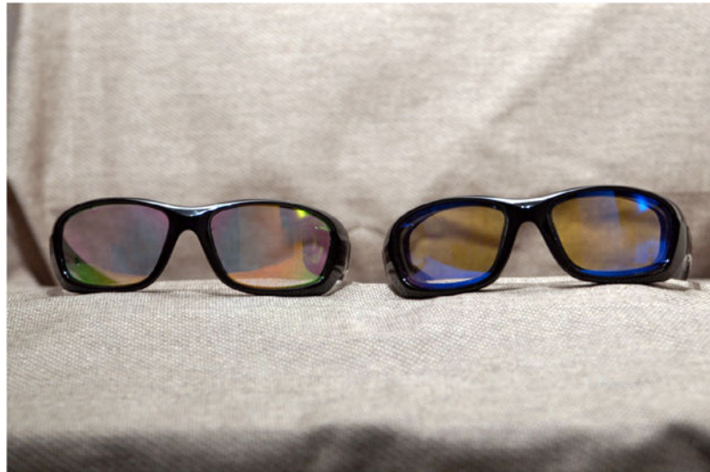
Fig. 2. Study glasses. Each subject initially was randomized to wear either a 480 nm optical notch filter lens (right) or a 620 nm optical notch filter lens (left).
